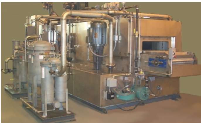
The lower photo shows a multi lane-multi stage belt washer for processing castings. Included are filtration systems for each spray pump, high pressure blow off system and a gas fired dryer.
