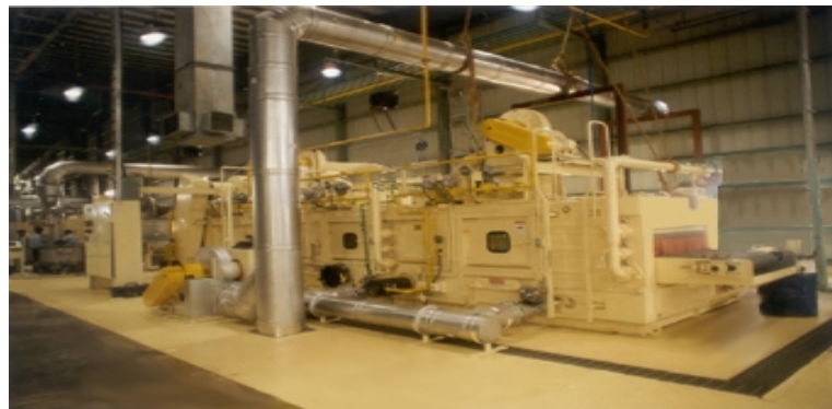
Center Photo (above) shows a multi-stage belt washer to thoroughly clean automotive radiator cores and heat exchangers prior to the application of solder flux. All equipment is furnished with stainless steel components.
